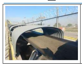
Copper concentrates on the PTFI Smelter conveyor belt being transported from the port to the Concentrate Barn. This concentrate is the product resulting from a process to separate copper from other minerals, with the concentrate subsequently undergoing refining at the PTFI smelter to produce pure copper.
